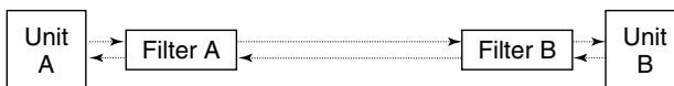
Figure 14.8 Scheme of two bidirectional coupled units A and B, each with a private commutative filter. From [27].
